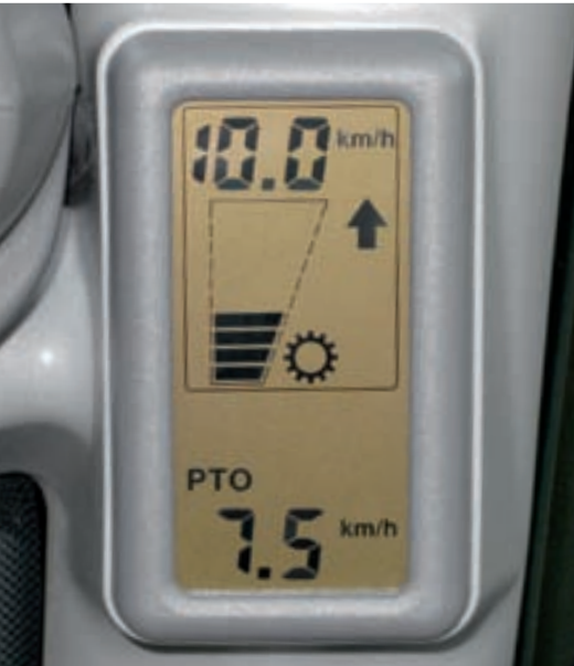
The transmission's PTO mode activates automatically when the PTO is switched on.
