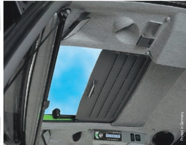
The tilting transparent roof has a ventilated, sliding sun-screen.
