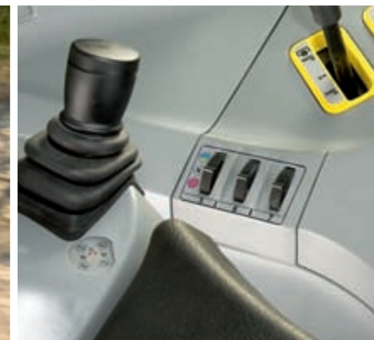
Up to seven remote valves can be operated (Agrotion TTV 630).
