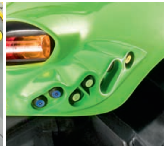
The powerlift can also be operated with the buttons on the mudguard.
