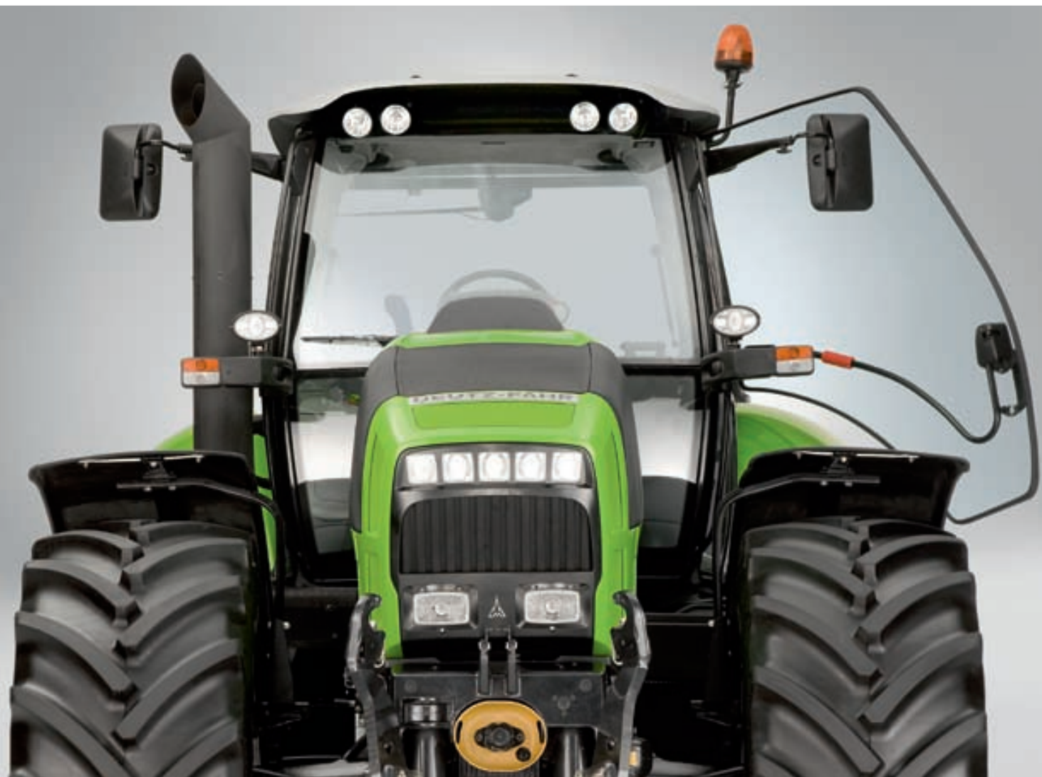
The front and rear windshields can be tilted fully (on the Agrottron TTV 630, just the rear windshield). And a large, tilting transparent roof is also included as standard.
