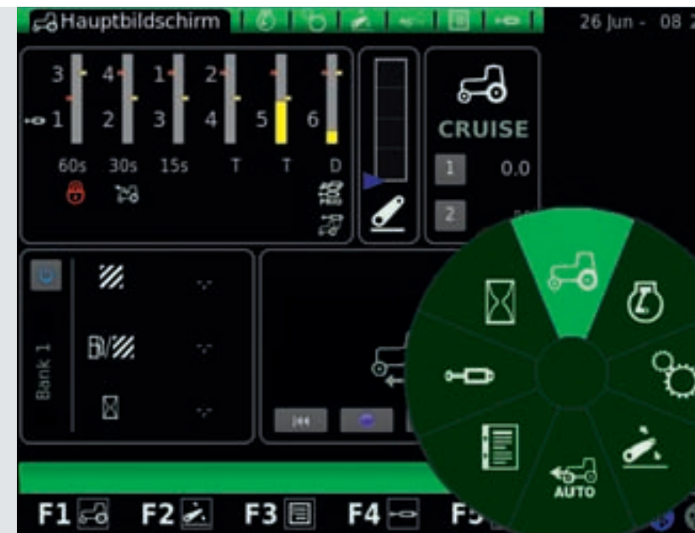
All important tractor functions are contained together in the main menu.
