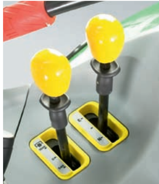
The PTO speeds can be conveniently pre-selected.
