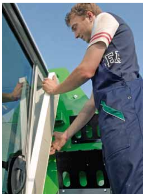
The cab air filter, a standard-feature, can be conveniently cleaned or replaced without tools.
