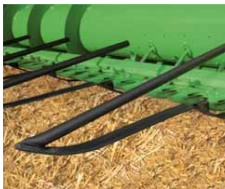
The standard ear lifters increase productivity with laid grain.
