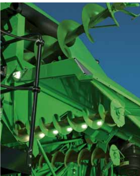
The grain tank discharge augers are pulled out to the side for servicing.
