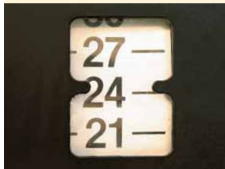
The threshing drum to concave clearance is shown in a window on the right-hand operating panel.
