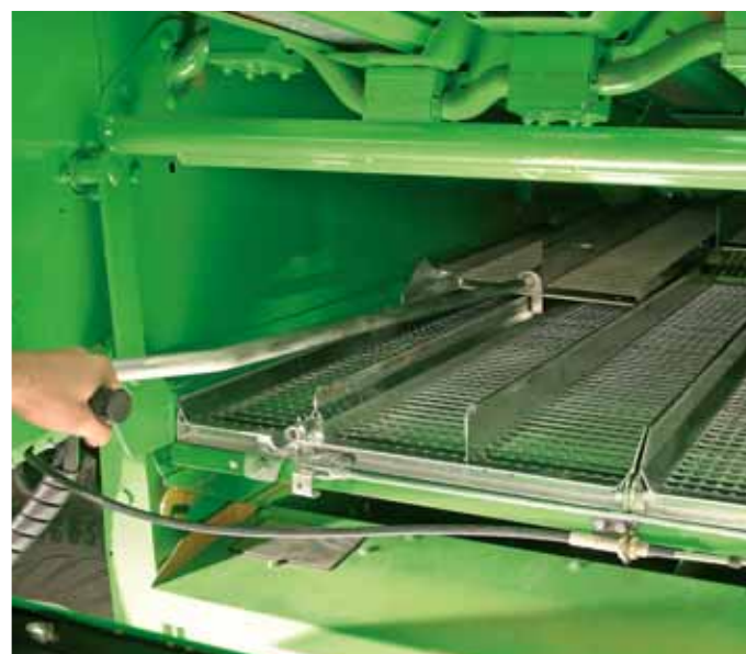
The individual elements of the preparation floor can be pulled out simply and conveniently for cleaning.
