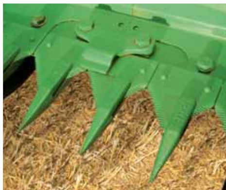
Robust fingers and serrated blades provide a clean cut.
