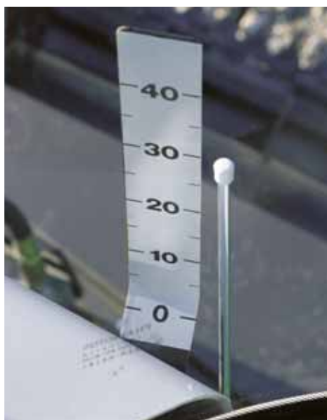
The cutting height display can be easily seen by the driver.
